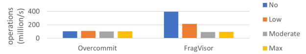
Figure 5. Operations per second achievable with Overcommit or FragVisor for different levels of concurrent writes.
